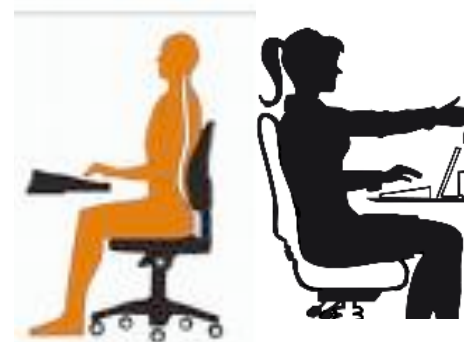
Classic 90:90 posture: back or shoulders cannot “rest” on the backrest; at 110° the back and shoulders can relax
